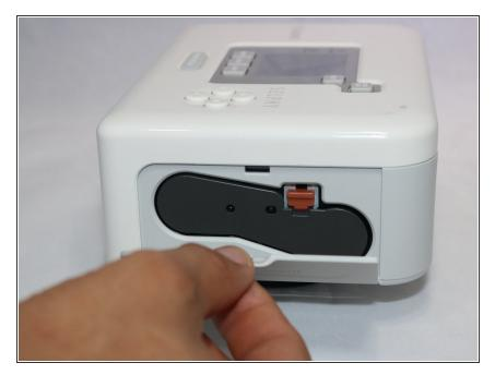
Pull open the top of the cover on the right hand side of the printer, so that the lnk Cassette is exposed.
