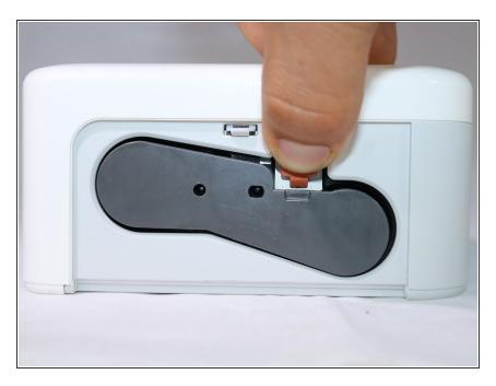
Lift the orange tab, which retains the Ink Cassette. If the Cassette is not jammed, it will eject automatically.
