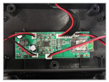
Remove the five wiring attachments (for the volume board, bluetooth board, speakers, and microUSB) from their connection to the motherboard by pulling slightly.
