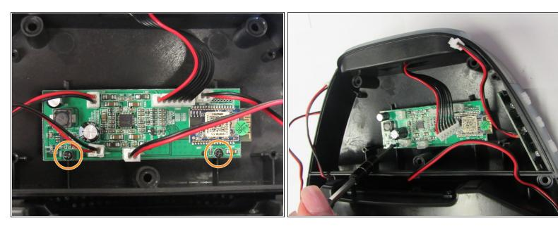
• Remove the two 9mm screws holding the motherboard in place using the Torx T5 screwdriver.
