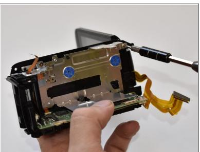
Remove the two 3mm Phillips #000 screws connecting to the display panel's hinges.
