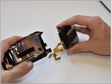
Remove the display panel by pulling the display straight away from the body.
