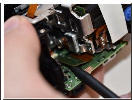
Using a spudger, disconnect the ribbon cable connector from the PC board shown in the picture.
