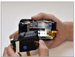
Using your fingers, firmly grasp both ends of the capturing device and gently pull the assembly straight out.
