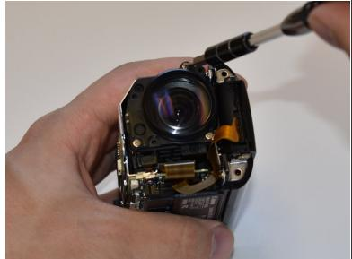
Remove the three 6mm Phillips #000 screws shown.
