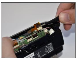
Using tweezers, disconnect this ribbon cable by pulling straight out.
