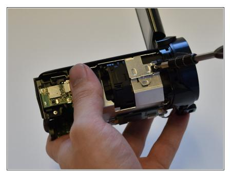
Remove the 5mm Phillips #000 screw on top of the inner case.
