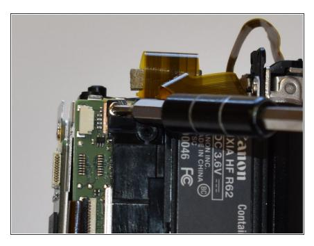
Remove the 4mm Phillips #000 screw at the bottom of the camera.
