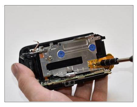
Remove the 3mm Phillips #000 screw holding the display's ribbon wire to the casing.
