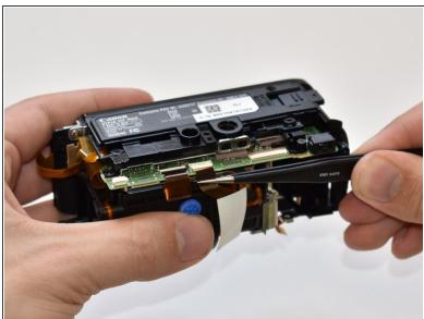
Using tweezers, disconnect the ribbon cable shown in the picture by pulling straight out.
