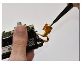
• The ribbon cable is also looped around a piece of the casing under the motherboard. Unfasten this cable with tweezers by sliding down and then pulling out.
