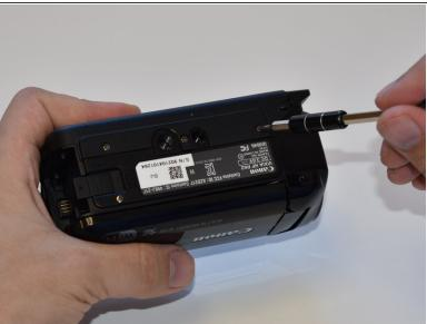
Remove the three 5mm Phillips #000 screws on the bottom of the device.
