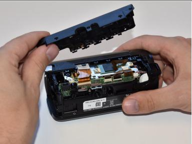
Remove the panel opposite the display by pulling up perpendicular to the side.
