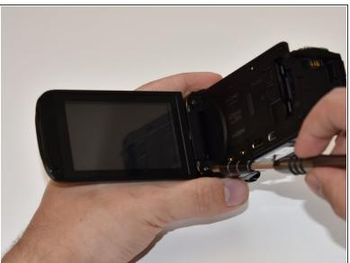
Remove the two 5mm Phillips #000 screws near the display panel.
