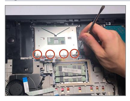
Remove the four 3mm screws using a Phillips #1 screwdriver in the locations shown.
