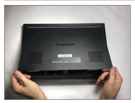
Remove the panel from the sides and pull it out at an angle towards you.
