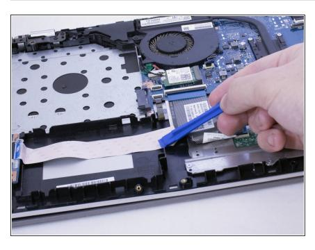
Use a plastic opening tool to pry the hard drive out.
