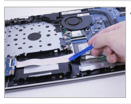
Lift the plastic wedges up on both sides of the hard drive.
