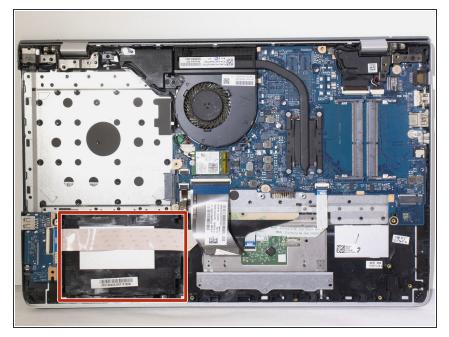
Use a spudger to lift the latch that holds the hard drive cable in place.
