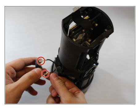
Pull on the speaker cables lightly in order to detach the speakers.
