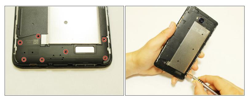
• Remove the seven screws using a Phillips #00 screwdriver.
