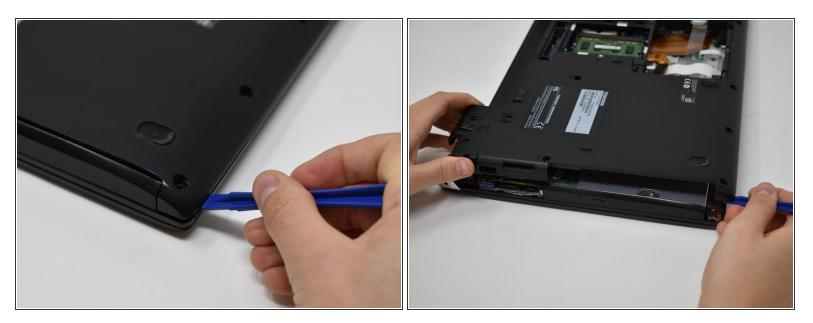
• Insert the plastic opening tool into the edge of the laptop and pry off the back cover.
