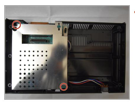
Remove the two 15 mm screws holding the casing in place using the Phillips #1 screwdriver.
