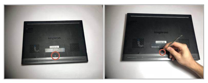
• Remove the 3mm screw in the location shown, using a Phillips #1 screwdriver.
