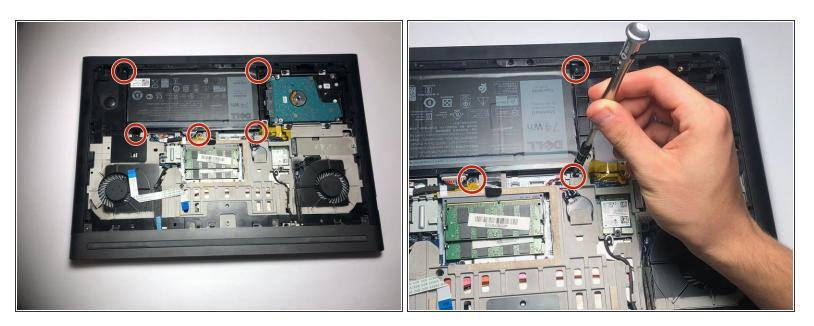
• Remove the five 3mm screws on the battery with a Torx (T8) screwdriver in the locations shown.
