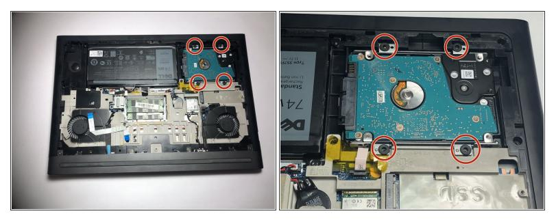
• Remove the four 5mm screws with a Phillips #1 screwdriver.
