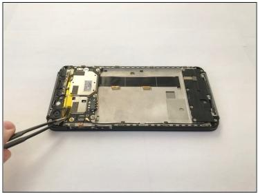
• Remove the yellow plastic tape using a pair of <u>tweezers</u>.
