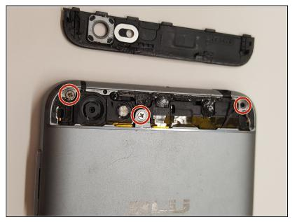
Using a Phillips #000 screwdriver, remove the 3mm screws. Be sure to do this for the top and bottom of the phone.
