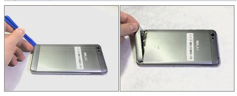
• Remove the two plastic plates with a plastic opening tool.
