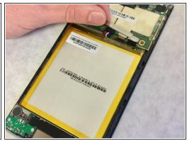
Use a driver with the T5 bit to remove the 3mm screws attaching the narrow metal plate to the main board.
