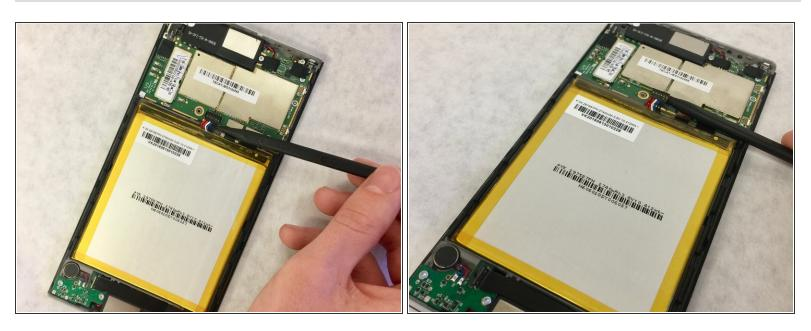
Slide the pointy end of the nylon spudger under the wires of the battery connector, and gently lift the wires away from the device, freeing the connector from the main board.
