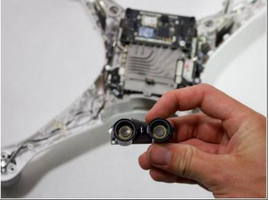
Pry the ribbon cable off the ultrasonic sensor using a plastic opening tool.
