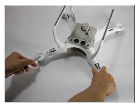
Pry the paper covering off the four corners with a metal spudger.
