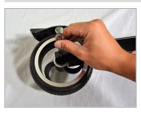
Flip over the scooter and use the hex bit 4.0 to remove the other 0.2 mm screw.
