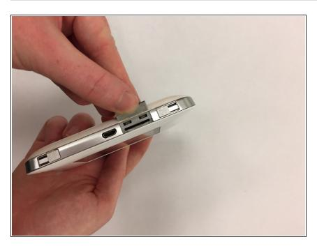
Look to the left of the charging port and peel back the SIM Card slot in order to open it.
