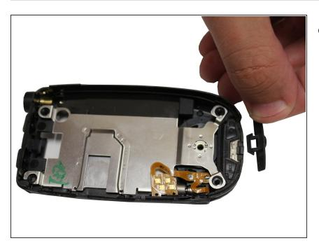
Once you have taken off the back cover of the phone, the charger tab can be lifted out of position on the back cover.
