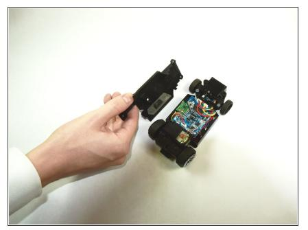
Remove the back-cover off and make sure there are no rust or disconnected wires.
