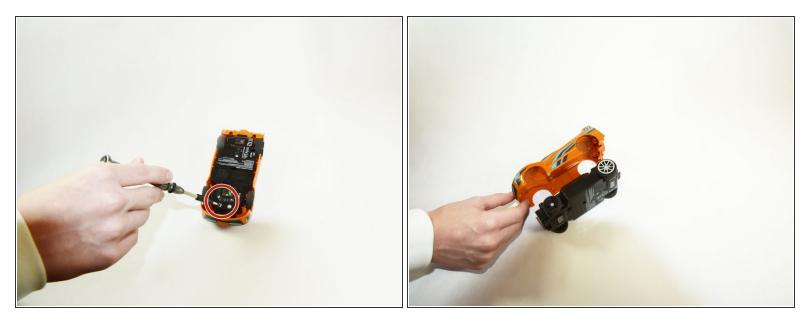
Locate the two screws on the back of the car towards the front. Use a #J0 JIS screw to loosen the screws.
