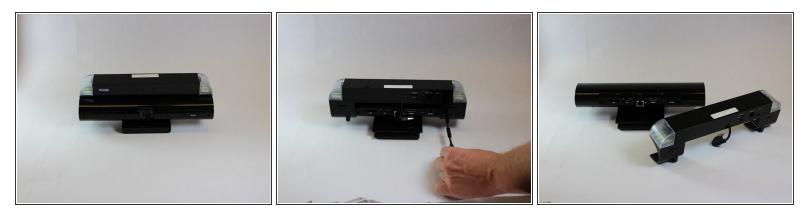
• Remove the top bar by removing the 5cm hex T10 screws on the back of the device as shown. Then gently pull off the top bar from the main component.
