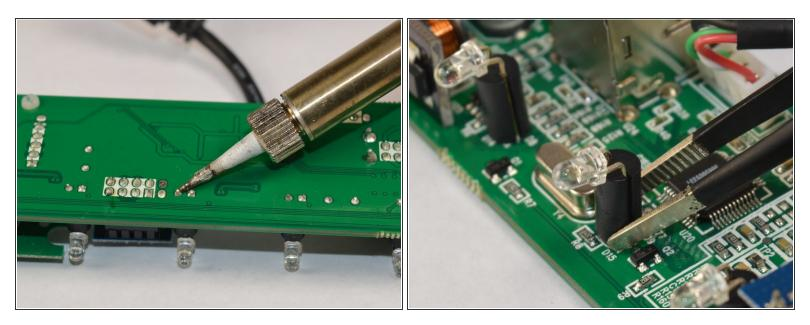
Heat the solder on the underside of the affected light to remove and replace it using tweezers.
