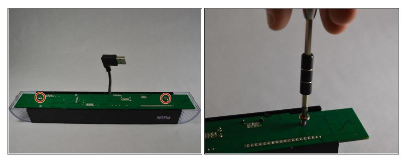
Remove the two 7mm screws holding the motherboard in place with a phillips head screwdriver size #00.
