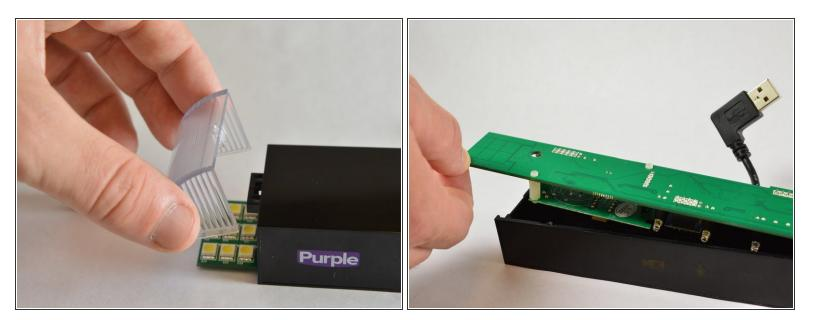
• To release the motherboard from its plastic housing, first pull the plastic light covers up and away from the device.
