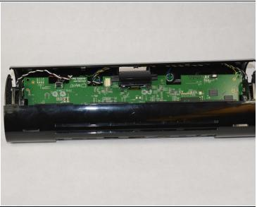
• Remove the 1.2 cm hex T9 screws and gently open up the device.
