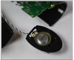
• Remove the speaker from the plastic shell of the device.
