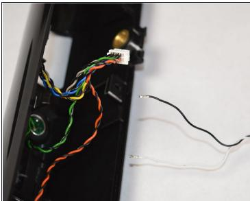
Release the wires connected to the speaker from the 12-pin connector with a spudger and replace the affected speaker.
