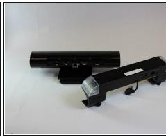
Remove the top bar by removing the 5cm hex T10 screws on the back of the device as shown.
