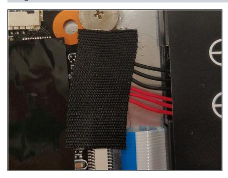
Remove the black adhesive strip covering the battery connector.
