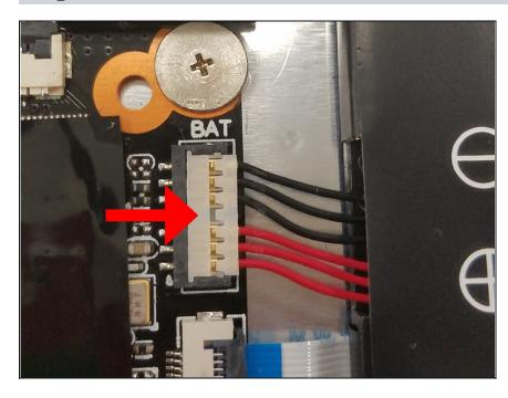
Gently remove the battery connector by slowly applying pressure on the connector in the direction of the battery.
