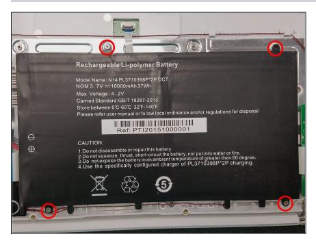
Use a J00 screwdriver to unscrew the 4 battery screws.
