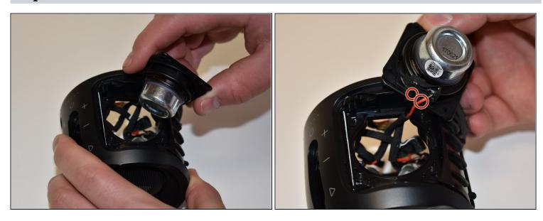
• Pull out the speaker and cut the black and red wire with wire cutters. The speaker should now be removed from the JBL Pulse 3.
