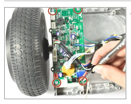
Remove the four 12mm Phillips #2 screws securing the sensor board.
