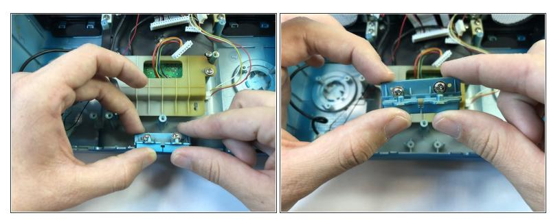
• Once the screws have been removed, simply lift the buttons up and out of their seat.
