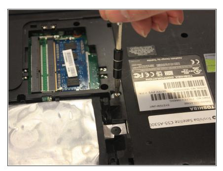
Remove the screw to the top right of the hard drive using the PH1 screwdriver.
