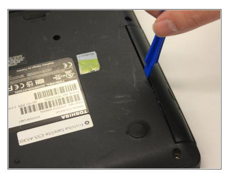
Use the plastic opening tool to wedge between the CD Drive and the laptop casing and gently pull it out.
