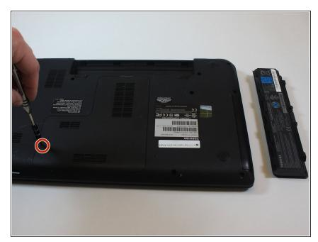
Unscrew the screw on the back panel of the laptop covering the hard drive.
