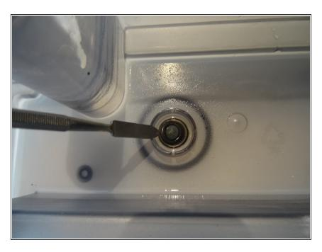
With your fingers press the valve stem from the bottom up. Now you can pry off the seal with a spatula tip.
