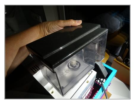
• Lift the water tank off the machine
