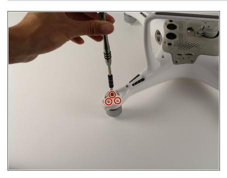
Remove the twelve 8.7 mm hex screws with a 2 mm hex bit from the motor bases.
