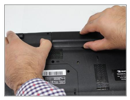
Pry the battery upward using the indent.
