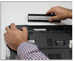
Continue to pull the battery until it is free of the casing.
