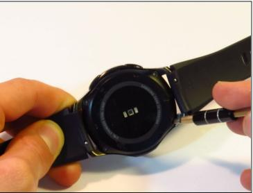
Remove the four 4.2mm screws with a Y00 screwdriver.
