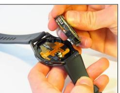
Separate the motherboard and front screen assembly using a spudger.
