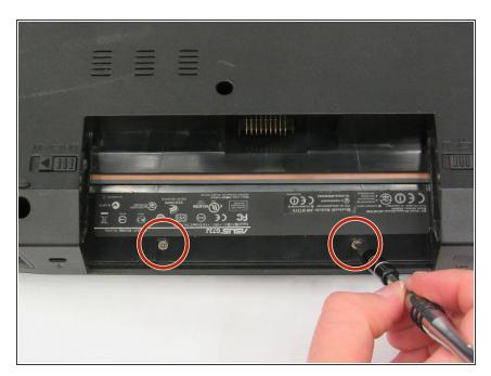
Remove the two 3 mm Phillips #0 screws in the battery port.
