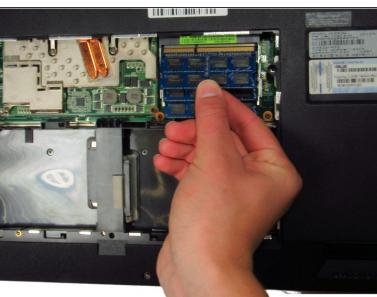
• Push the metal retaining arms away from RAM cards. One edge of the card should release and stick upwards at a 30 degree angle. Grab the free edge of the RAM card with your fingers and pull it free. Repeat this process with the following two cards.
