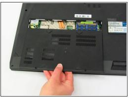
Insert the plastic opening tool into the small groove at the edge of the panel. Using the plastic opening tool, gently pry the back panel upward until it lifts free from the device. Gently lift the panel away with your fingers.
