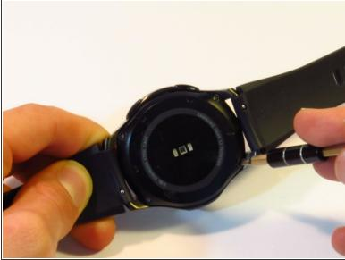
Remove the four 4.2mm screws with a Y00 screwdriver.
