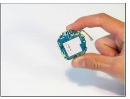
Remove the battery's cable from the chassis using tweezers.
