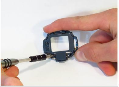
Remove the single 3.9mm screw with a JIS #000 screwdriver.
