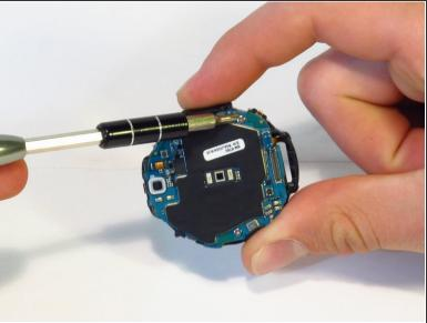
• Using a JIS #00 screwdriver, remove the two 4.5 mm screws.
