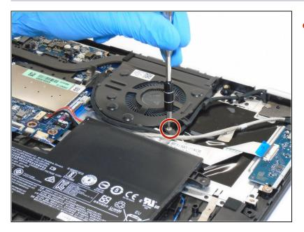
• Remove all screws securing the fan to the laptop.
