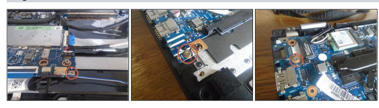
• After the flap is opened then you will have to go and remove all the screws holding the circuit board to the computer.
