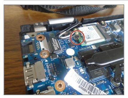
After the screws are removed from the circuit board, you will have to remove these last screws to remove it completely.
