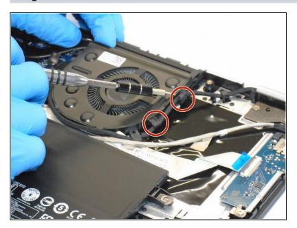
Unhook the wire from the fan component using a spudger.
