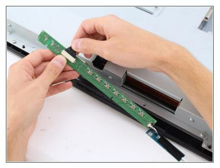
Remove the button board by pinching the wiring close to the connector and gently pulling straight out from the port.
