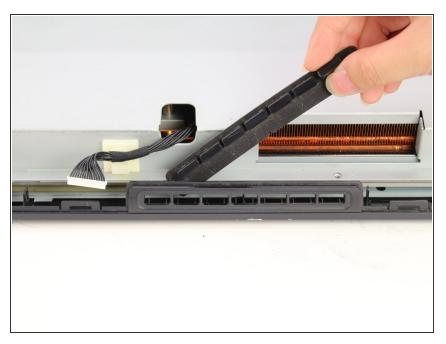
• Remove the button cover by pushing the buttons out of their holes and pulling the cover up.
