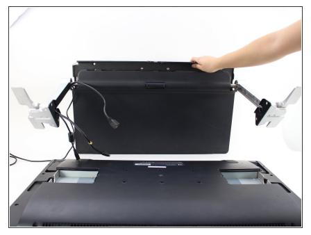
• Lift the stand up and away from the rest of the device so the legs separate from the mounting plate.
