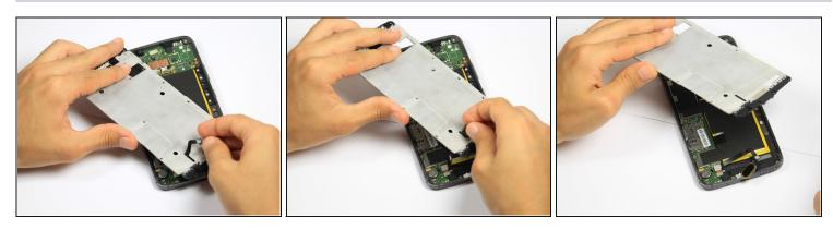
• Grab ahold of the fingerprint sensor and push it through the opening in the metal cover.
