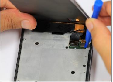
• Disengage the two cable connectors by gently prying beneath the edge of the connector with the opening tool.
