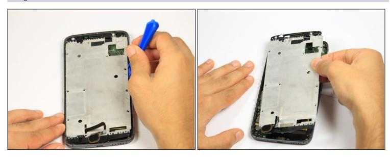
• Remove the metal cover by prying underneath it with the opening tool.
