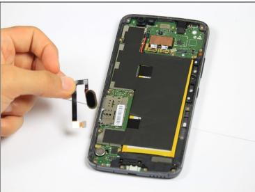
Remove the fingerprint connector by gently prying underneath the connector with the opening tool.
