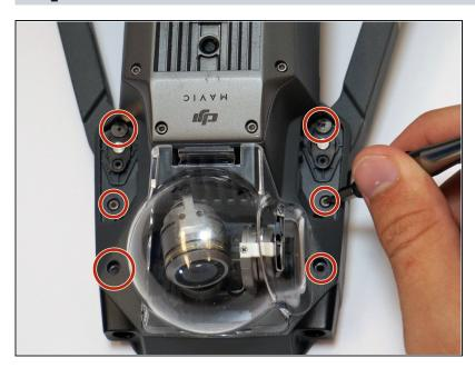
Remove the six 5mm 1.5 Hex screws that are under the panel pieces by turning the screwdriver counterclockwise.
