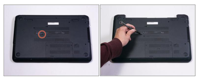
Use a J1 or PH1 screwdriver to remove the 6.5mm screw that secures the optical drive.
