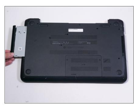
• Gently remove the optical drive once it has been loosened.
