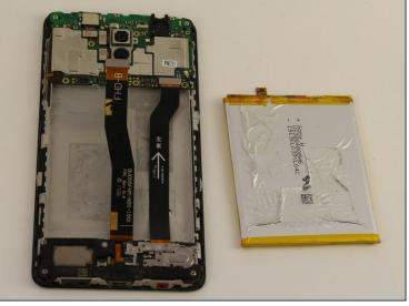
• Using the <u>plastic card</u>, remove the battery by lifting it from the casing.
