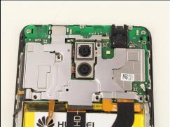
• Remove the five 4mm Phillips #00 screws using a screwdriver.
