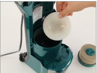
• Pull out the felt filter from where the foam filter rested.
