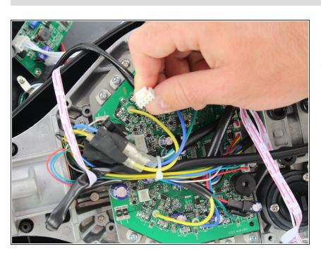
Remove the charging port connector from the motherboard by squeezing the connector and pulling the connector up.
