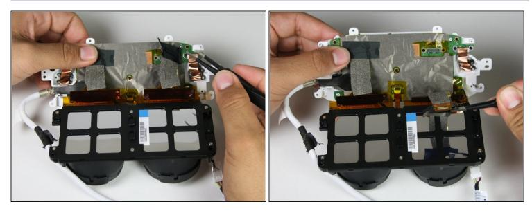
• Take off the tape using the blunt nosed <u>tweezers</u> to disconnect the flat-topped connector from the motherboard.
