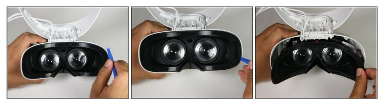
• Remove the cover using one of the plastic opening tools, and then carefully pull it from the casing.
