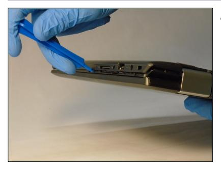
• Pop off the back panel using a plastic opening tool once all screws are removed.
