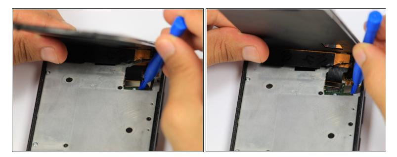
• Disengage the two cable connectors by gently prying beneath the edge of the connector with the opening tool.
