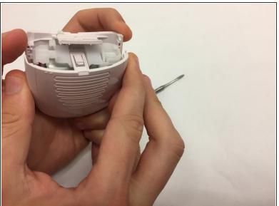
• Use a metal spudger to pry open the casing.
