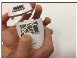
Remove the head by pushing it to the right.
