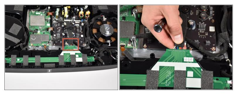
• Disconnect the main speaker array from the main board, by pinching and and pulling the tab out.
