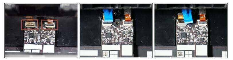
• Remove ZIF connectors by lifting the black tabs and pulling the ribbon out.
