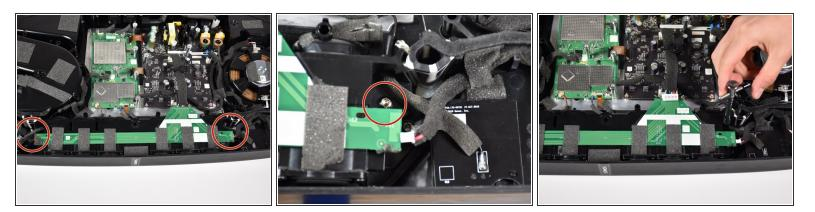
Remove the two 16mm <u>T-20</u> screws located on both sides of the main speaker array by turning counter-clockwise.
