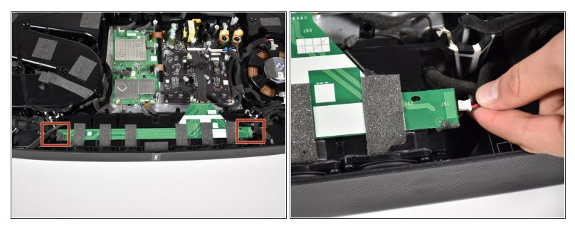
Remove the side speakers from the green printed circuit board (PCB) running along the top of the main speaker array by pinching and pulling out the connector.
