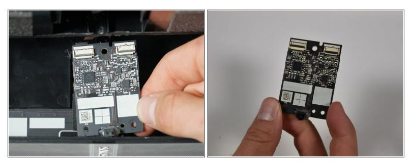
• Remove the IR receiver by grasping it with two fingers and pulling up.
