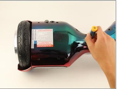
Remove the two 11mm Phillips #1 screws that hold the base plate to the body.
