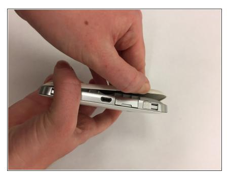
Using your finger, pry open any of the four corners of the back of your AirCard 770S, until you see the back case disconnect from the device.
