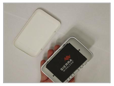
• Lift open the back case and remove it from the device.
