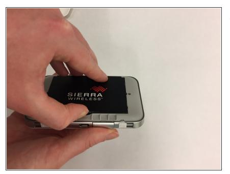
With the bottom of the device (above the charging port) facing you, use your thumb nail to lift up the battery.
