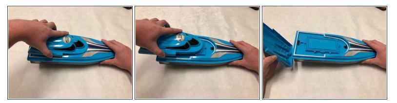
• Remove the top of the boat by sliding it backwards and then pulling it off.
