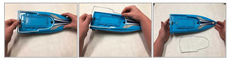
• Gently remove the gasket and replace with a new one.
