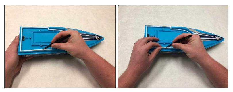
• Grab the rubber gasket with tweezers and pull it out of the slot.
