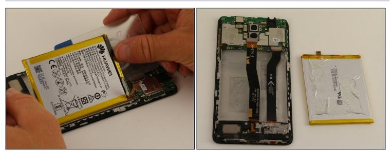
• Using the <u>plastic card</u>, remove the battery by lifting it from the casing.
