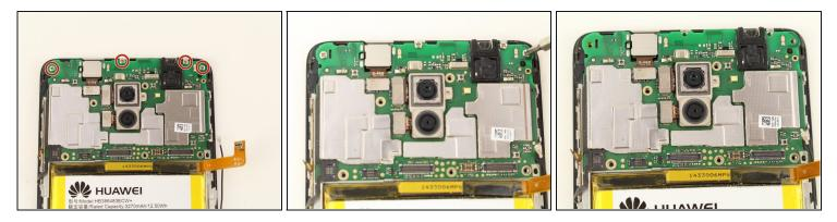
• Remove the four 2mm Phillips #00 screws.
