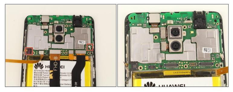
• Remove the last two connectors from the motherboard using a spudger or your fingers.
