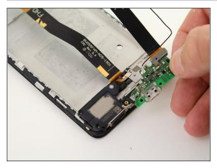
• Pry the micro USB port off of the phone using a spudger.
