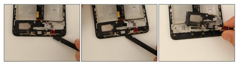
• Pry the speaker and microphone assembly off of the phone by sliding a spudger down along the bottom.
