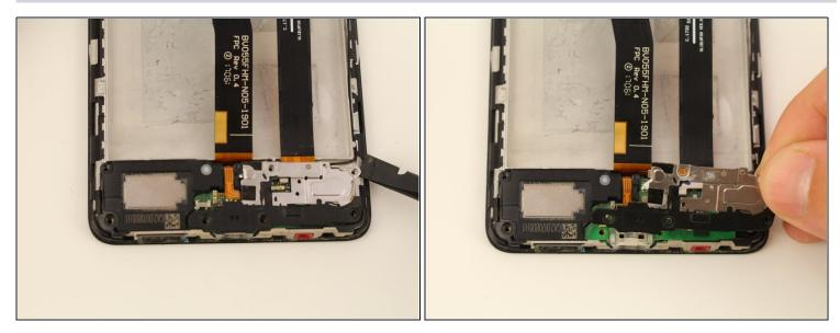
• Remove the metal plate from the vibrator assembly using a spudger.
