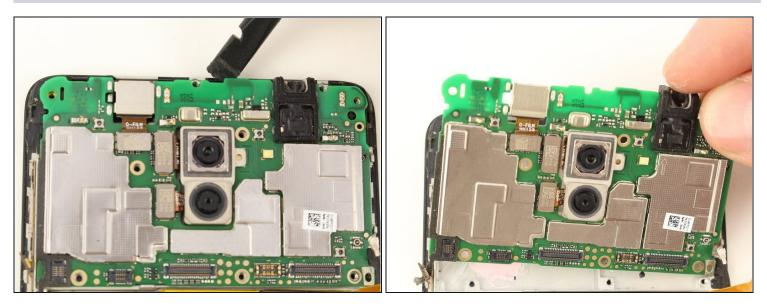
• Gently lift the motherboard from the phone using two fingers or a spudger.
