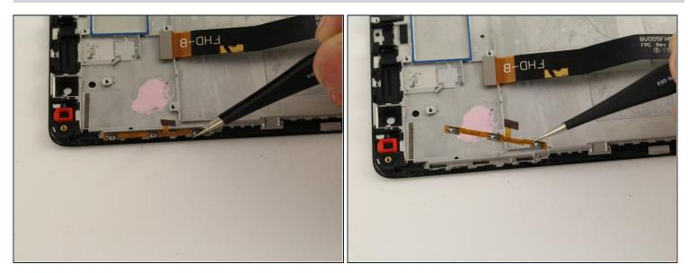
• Pull the volume buttons off using tweezers or the end of a spudger.
