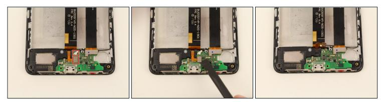
• Snap the two connectors off using a spudger or your finger.
